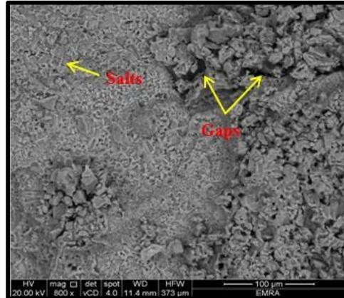
**Fig. 9:** SEM photomicrograph of the second sample shows the presence of quartz grains, the spread of gaps and the crystallization of salts under magnification (800X).
