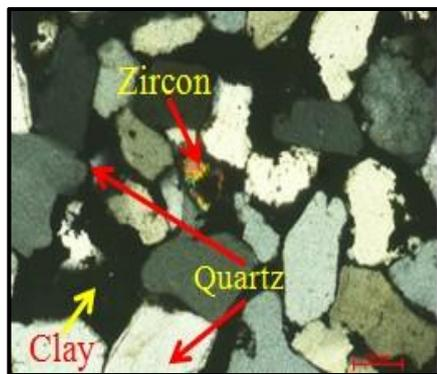
Fig. 6: Petrographic micrograph of the second sample in south Sinai shows the presence of monocrystalline quartz grains, iron oxides and zircon grains under magnification (10 X - CN).
