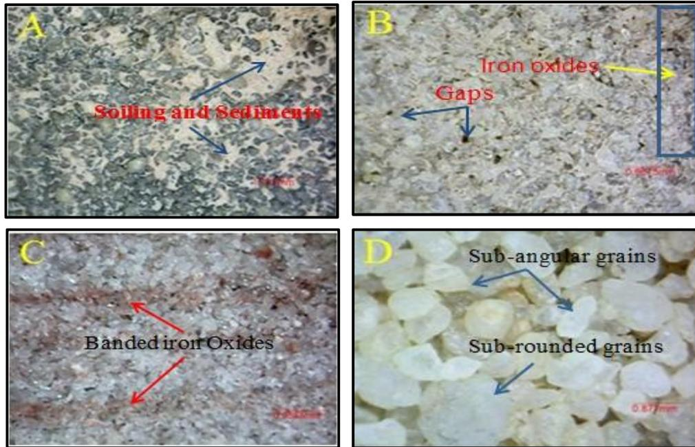
**Fig. 4:** Microphotograph Usb stereo-microscope of sandstone sample In Wadi Nasib A: Quartz grains " Arenite" and sand deposits, B: quartz grains " Arenite ", iron oxides and some gaps C: banded iron oxide D: various quartz grains.
