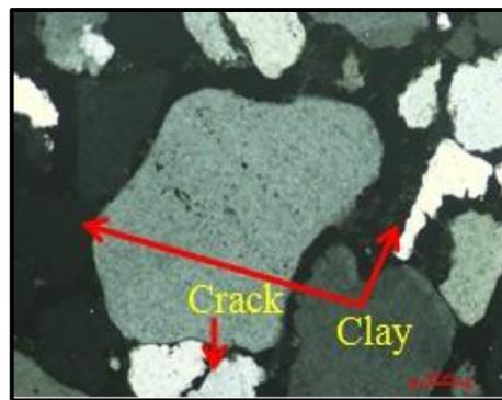
Fig.7: Petrographic micrograph of the same second sample showing presence of quartz granules, clay minerals as cementing material and some cracks under magnification (10 X-CN)
