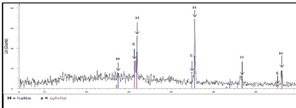
Fig. 15: Represents XRD pattern of the third sample in Wadi Nasib, South Sinai.
