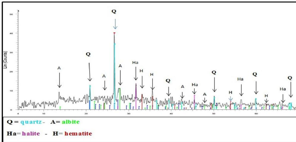
Fig. 14: Represents XRD pattern of the second sample in Wadi Nasib, South Sinai
