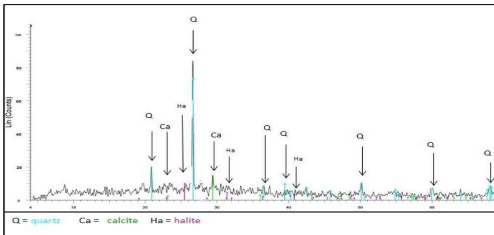
Fig. 13: Represents XRD pattern of the first sample in Wadi Nasib, South Sinai
