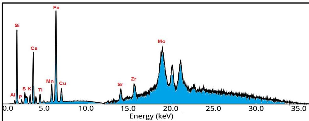
**Fig. 11.** Represents XRF pattern of the first sandstone sample in Wadi Nasib in south Sinai
