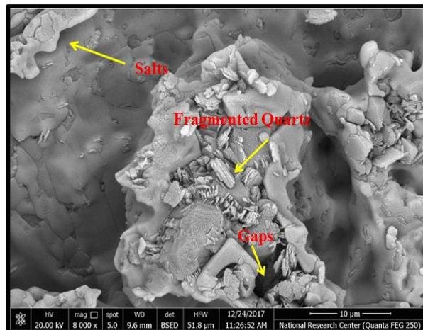
**Fig. 10:** SEM photomicrograph of saline sample in Wadi Nasib in Sinai shows the presence of the phenomenon of fragmentation and gaps and salt crystallization (8000 X).
