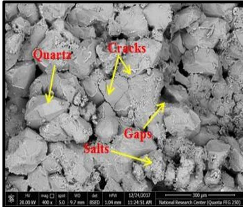
**Fig. 8:** SEM photomicrograph of the first sandstone sample in Wadi Nasib Sinai shows the existence of quartz grains, some gaps and cracks under magnification (400 X).
