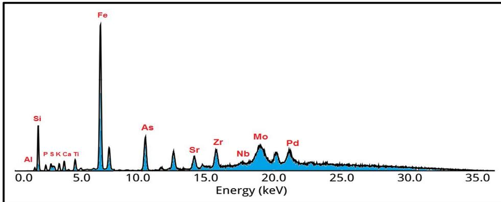
Fig. 12: Represents XRF pattern of the second sandstone sample in Wadi Nasib in south Sinai
