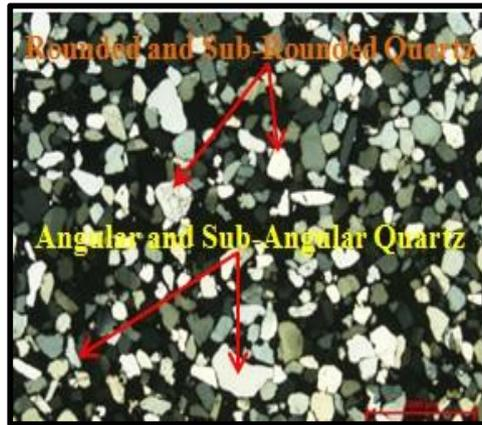
Fig. 5: Petrographic micrograph of the first sample showing presence of round, sub-round and angular quartz grains of different shapes and sizes, (10 X - CN).
