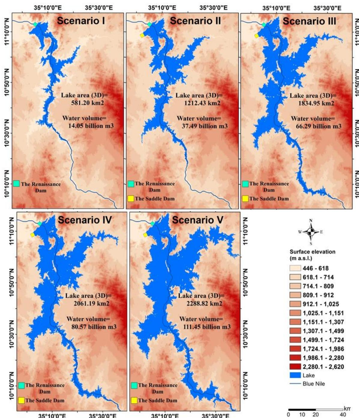
**Fig. 3:** The reservoir of the Renaissance Dam under five scenarios of Dam altitude i.e. 88 m (scenario I), 117 m (scenario II), 137 m (scenario III), 145 m (scenario IV) and 170 m (scenario V).
