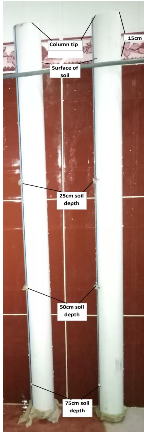
Fig. 2: The apparatus used in studying slow release fertilizer behavior compared to control
