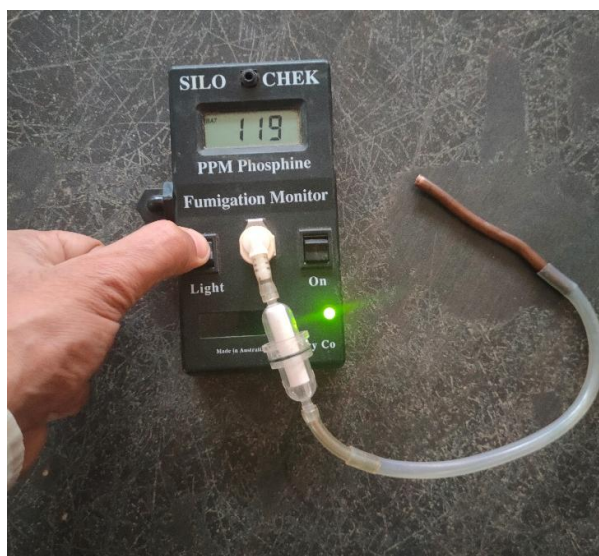
Fig. 2: Silo-Check device for measuring the concentration of \text{ECO}_2 -Fume gas inside a pile
