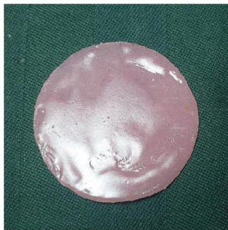
Fig. 2: Heat-cure specimen relined with resilient liner.
