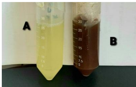
Fig. 1: Show change in color of fruit extract from yellow to yellowish brown (A) citrus paradisi fruit extract, (B) biosynthesized silver nanoparticles at 60°C.
