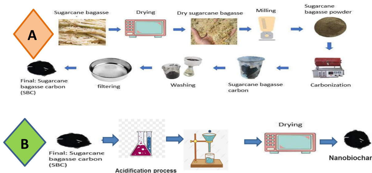
Fig. 1: Preparation of biochar and nanobiochar from bagasse
