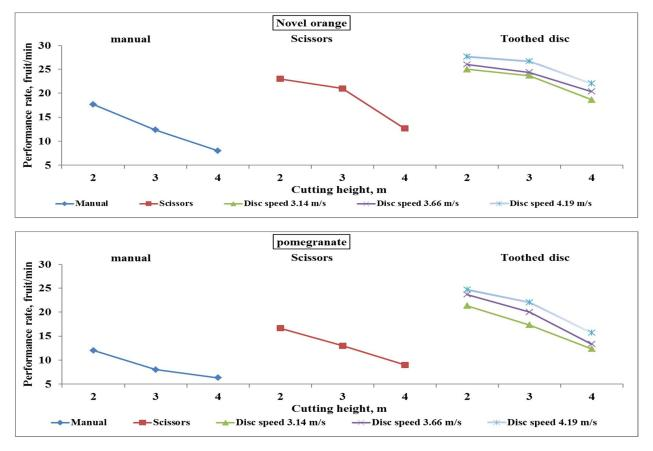
Fig. 6: Effect of some operating parameters on machine performance rate for harvesting navel orange and pomegranate fruits
