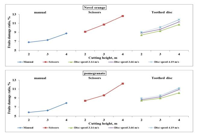
Fig. 7: Effect of some operating parameters on fruits damage ratio for harvesting navel orange and pomegranate fruits
