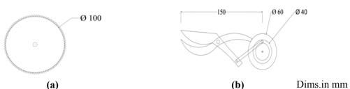
**Fig. 3:** Schematic views of the different cutter head types: (a) toothed disc (b) scissor
