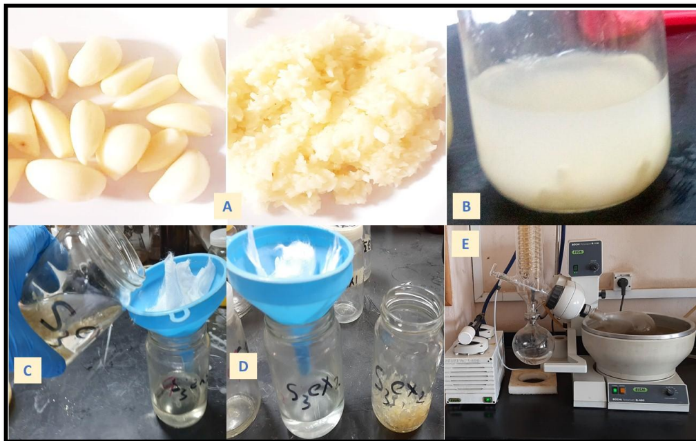
Fig. 1: Steps for preparing the garlic extract, A: grinding the garlic cloves, B: mixing the crude extract with solvent after gently shaking for 48 h, C&D: filtration, and E: solvent removal by rotary evaporator.
