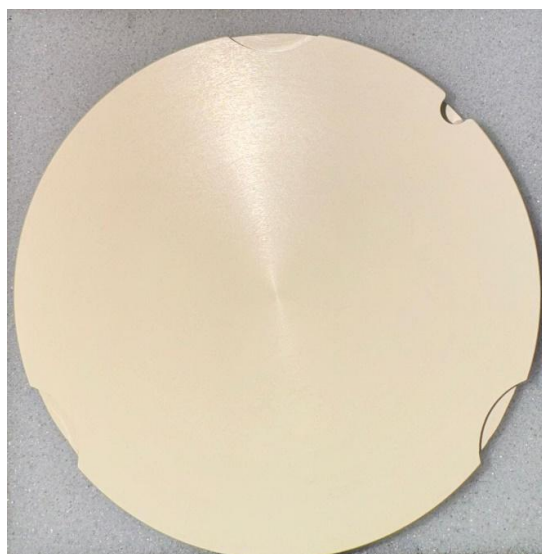
Fig. 1: PEEK Disc used for milling PEEK post and core
