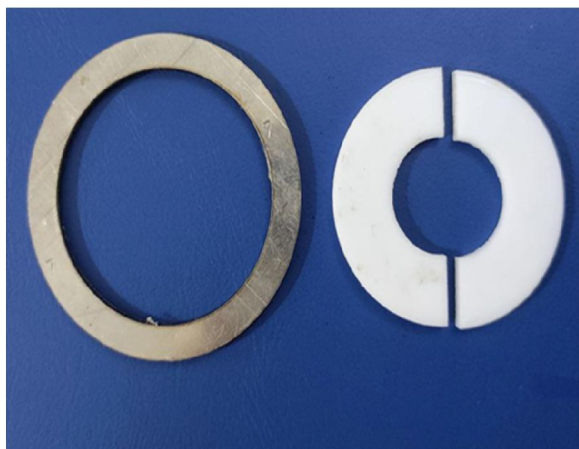
Fig. 1: Showing push out bond strength mould.
