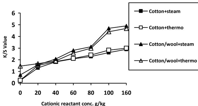
**Fig. 1:** Effect of Sera Fast C-B concentration (using steaming or thermofixation after cationisation) on K/S values of dyed cotton and cotton/wool fabrics with the reactive dye.
