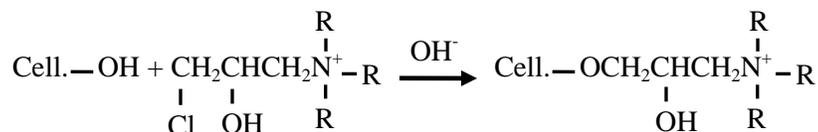
**Scheme 1:** Cationically modified cotton when a cationic reactant reacts with cellulose under alkaline conditions.
