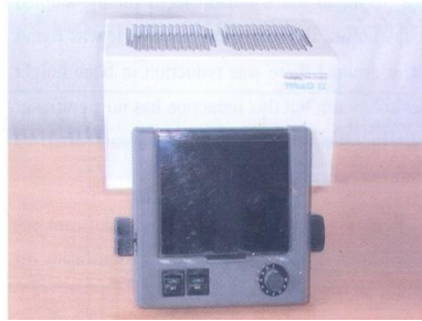
Fig. 4: The visible light curing unit
