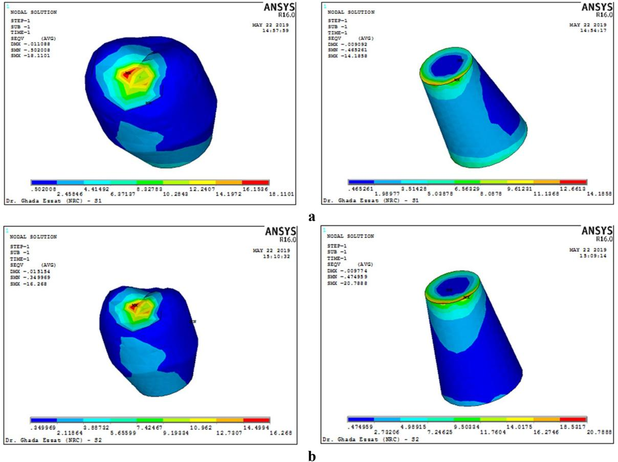
**Fig. 3:** Von Mises stress distribution on crown and cement;
