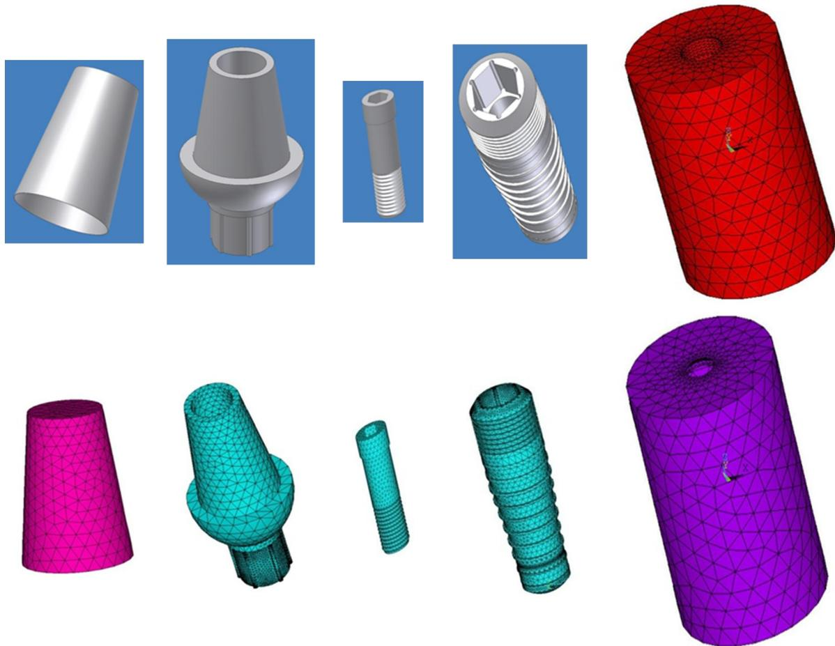
**Fig. 2:** Modeled and meshed model components
