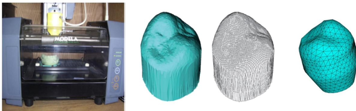
**Fig. 1:** 3D scanner and resultant surface after trimming and volume meshing
