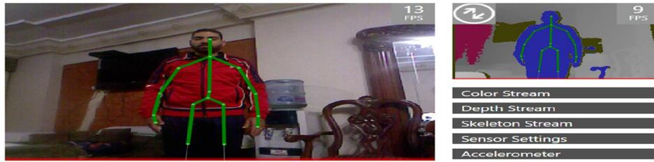
**Fig. 9:** Represent Microsoft kinect recognition when a person about 0.5 meter distance
