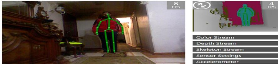
**Fig.10:** Represents Microsoft kinect recognition when a person at around 4 meters distance
