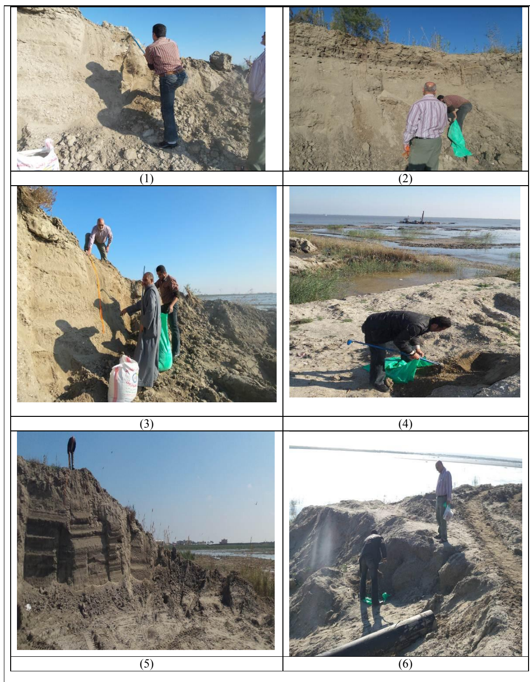
Fig. 3: Stages of samples collections. (1) Crushing from top to bottom. (2, 3,4,5) Collecting of samples. (6) The height of the production accumulation section.
