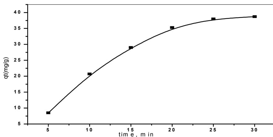
Fig. 3: Effect of contact time on the uptake of Fe (III) at 410.4 mg/l and 22°C
