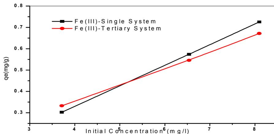
**Fig. 17:** Effects of different concentrations of Fe(III) in single and tertiary systems on ferric uptake
