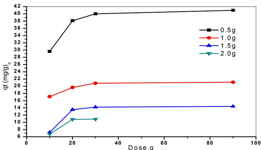
Fig. 2: Effect of the resin dosage on the ferric uptake
