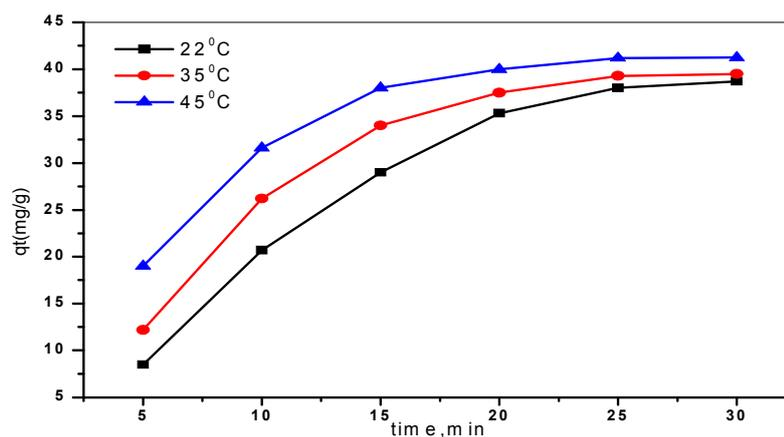
Fig. 14: The temperature effects on the uptake of ferric ions
