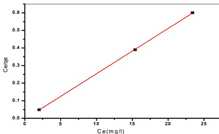
**Fig. 7:** The Langmuir plot of ferric adsorption
