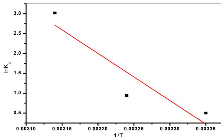
**Fig. 15:** The Van't Hoff plot of ferric adsorption
