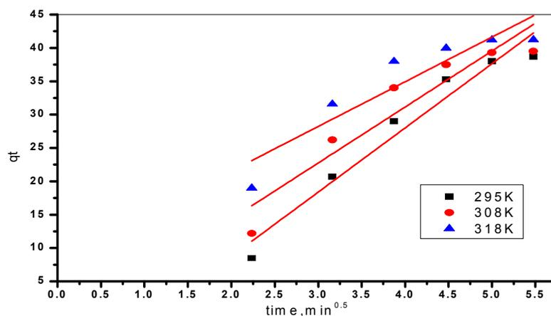
**Fig. 12:** The Intra-particle diffusion plot of ferric adsorption
