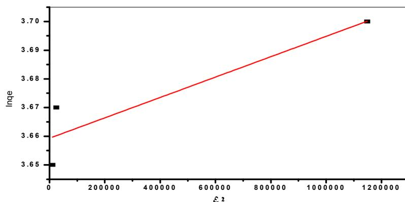
**Fig. 9:** The D-R plot of ferric adsorption
