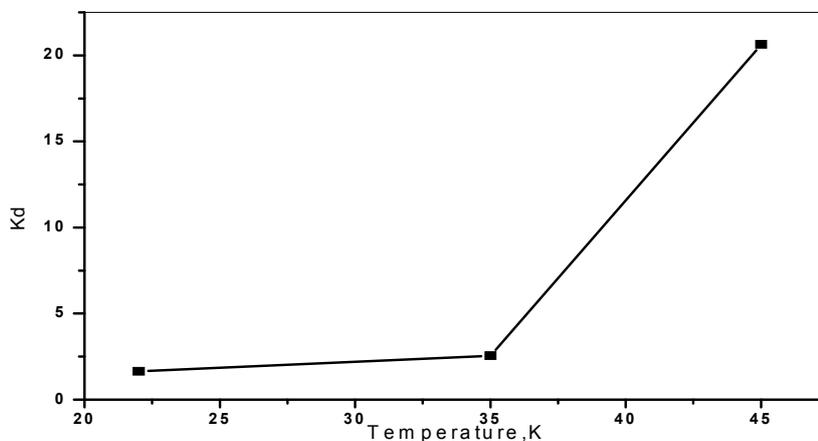
**Fig. 5:** Distribution coefficients of ferric at different temperatures
