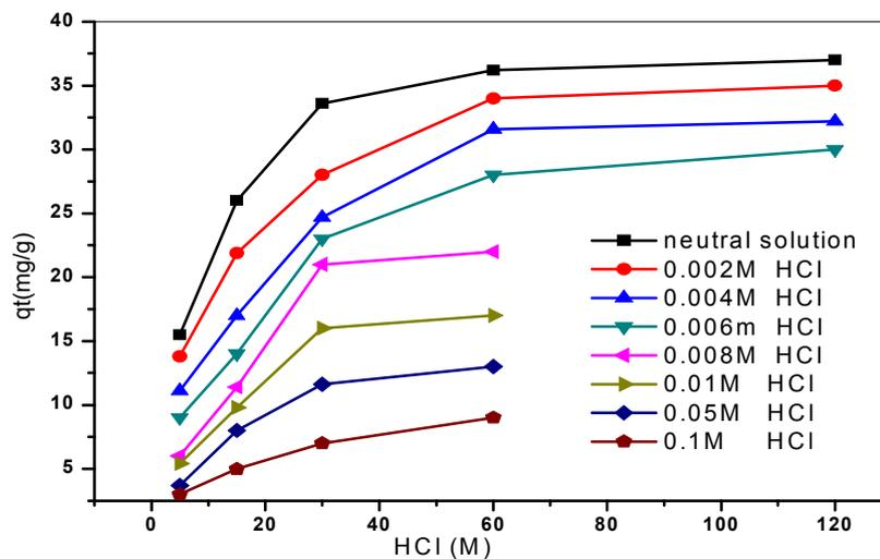
**Fig. 4:** Hydrochloric acid effects on the ferric uptake at 430.35 mg/l and 22°C
