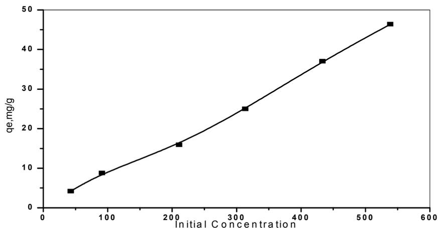
Fig. 1: Effect of different initial ferric concentrations on the maximum uptake
