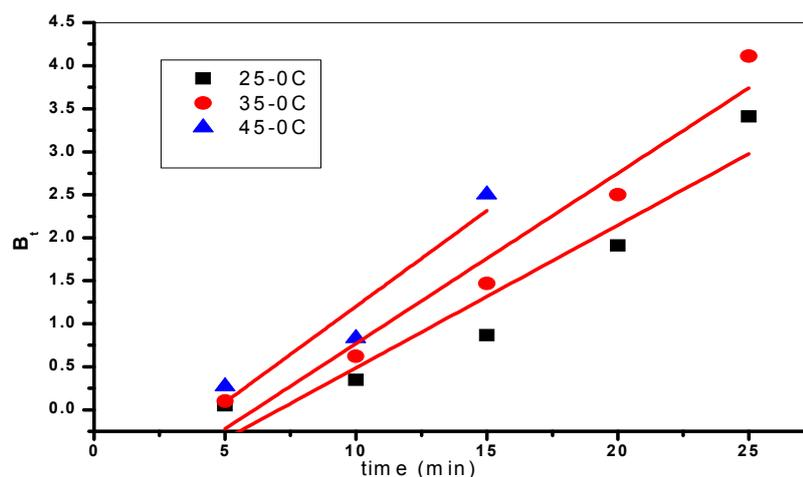
Fig. 13: Boyd plot for Fe (III) adsorption at 0.5g/50ml, 410.4 mg/l and at different temperatures
