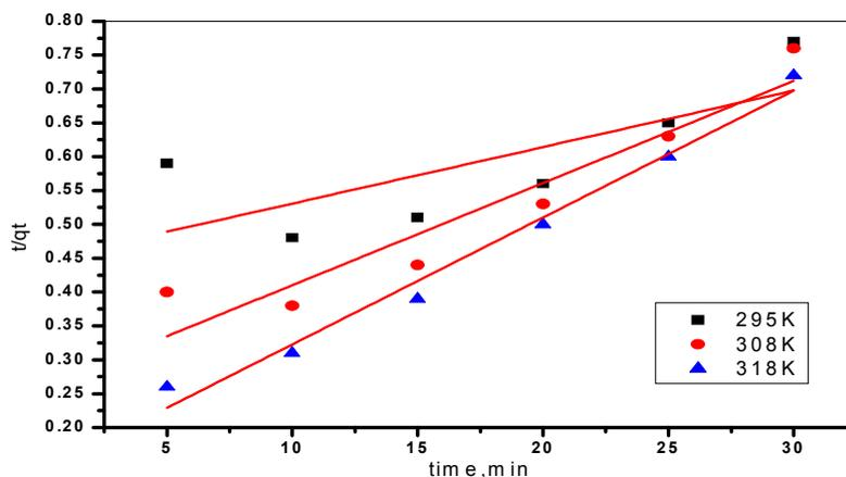
**Fig. 11:** The Pseudo-second-order plot of ferric adsorption at different temperature
