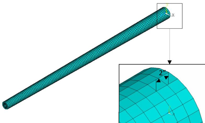
**Fig. 2:** Finite Element Meshing of the Pole in the Longitudinal Direction
