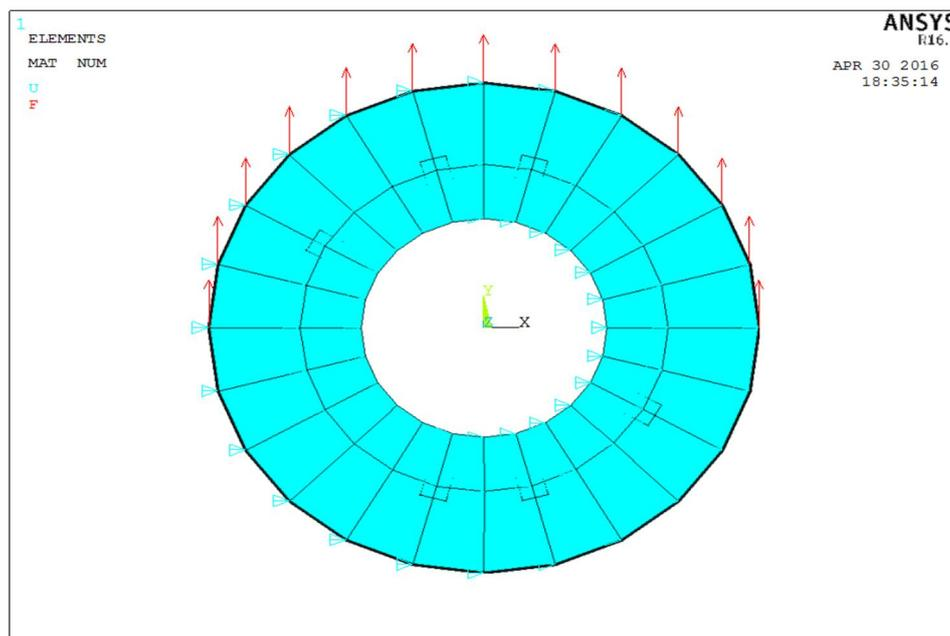
**Fig. 6:** Point loads applied to the pole
