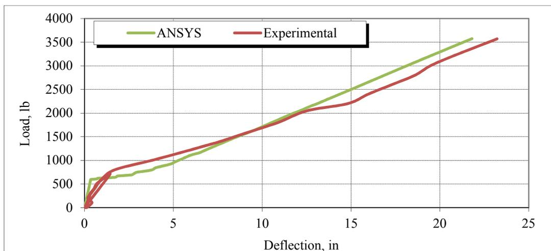
**Fig. 8:** Load-deflection curve for the second pole
