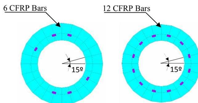
**Fig. 3:** Finite Element Meshing of the Pole in the Cross-sectional Direction
