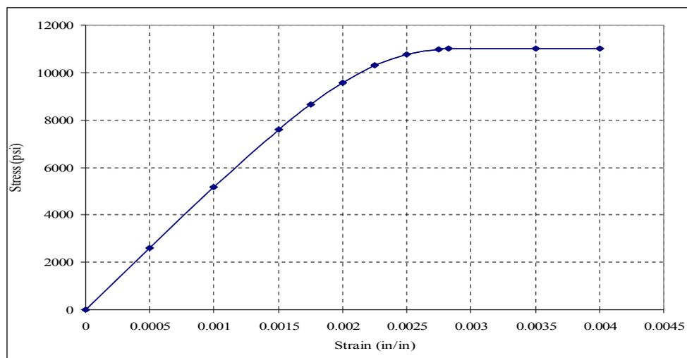
**Fig. 1:** Concrete stress-strain curve adopted in the FE model
