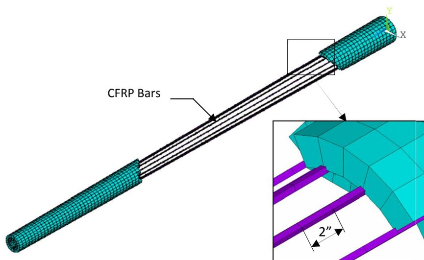
**Fig. 4:** Finite Element Modeling of the CFRP Bars
