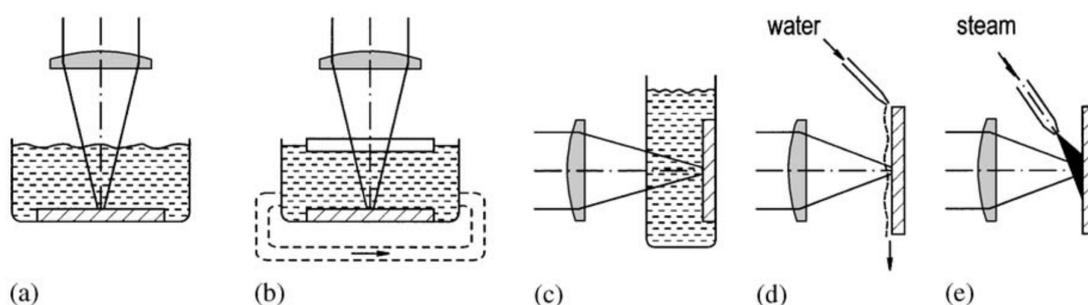
**Fig. 1:** Methods for providing water in the working zone during laser etching. Sources: (a) (Corbierre *et al.*, 2006); (b) (Yin *et al.*, 2004); (c) (Link and El-Sayed, 1999); (d) (Jain *et al.*, 2007); (e) (Corbierre *et al.*, 2006). In the cases (d) and (e), laser light not well transmitted by the water can be used. The thickness of the liquid layer over the target has typically been 1 mm:
