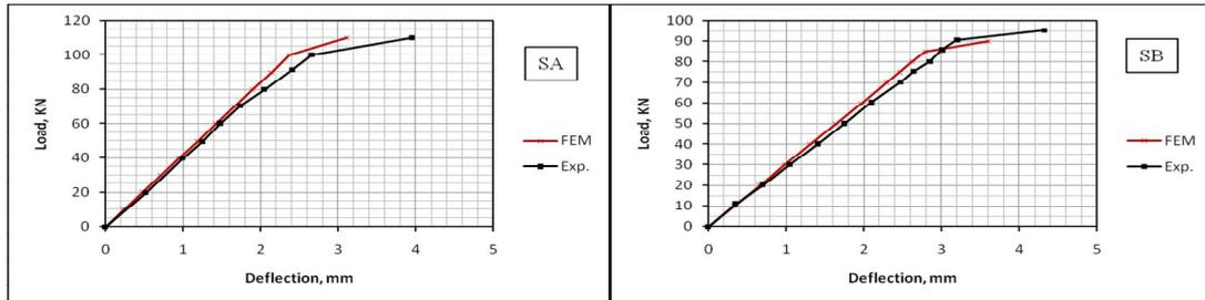
**Fig. 12:** Load-deflection curves for slabs SA and SB (At point A of max. deflections).
