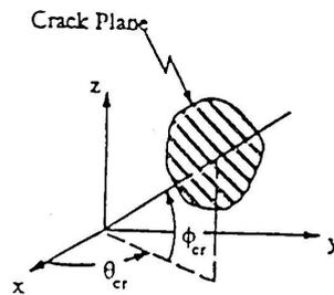
Fig. 6: Cracking plane in (Solid 65).
