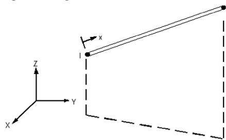
**Fig. 7:** Geometry, node location, and coordinate system of 3-D spar element (Link 8).
