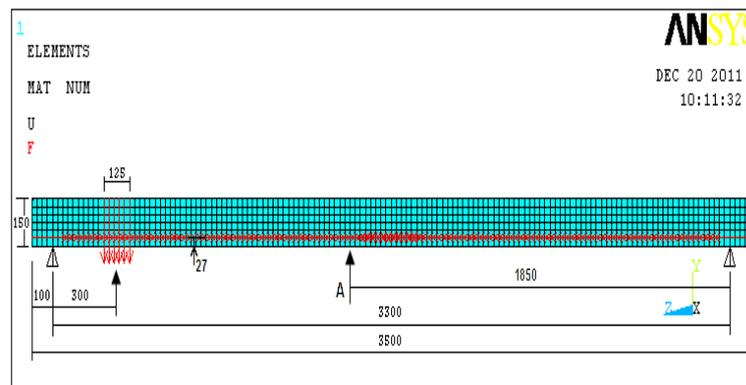
**Fig. 10:** Points of recorded deflection (Under vertical load and at point A).
