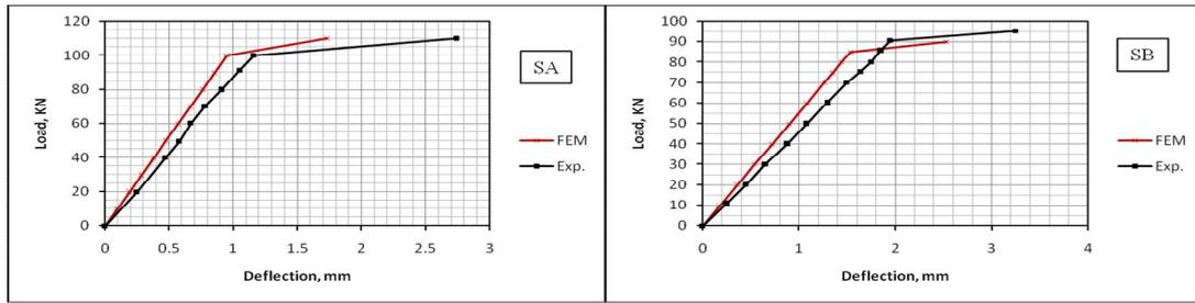
**Fig. 11:** Load-deflection curves for slabs SA and SB (At point under vertical load).
