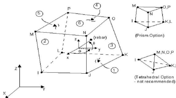
**Fig. 4:** (Solid 65) 3-D concrete element.
