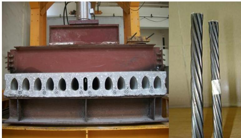
**Fig. 1:** Nominal cross-sections for test slabs and seven-wire prestressing strands.
