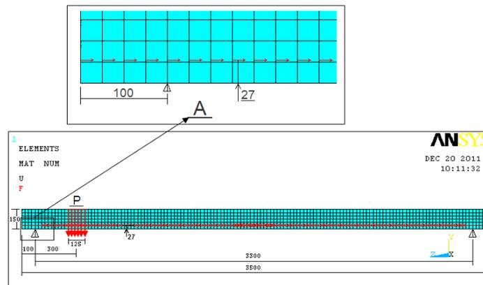
**Fig. 8:** Finite element model for pre-stressed hollow core slab (Show applied prestressing load).
