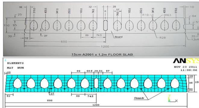
**Fig. 9:** Typical dimensions of the cross-sectional area and strands.
