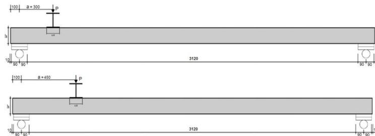
**Fig. 3:** Loading of slabs SA and SB.
