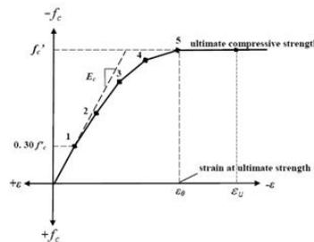
Fig. 5: Simplified compressive uniaxial stress- strain curve of concrete.
