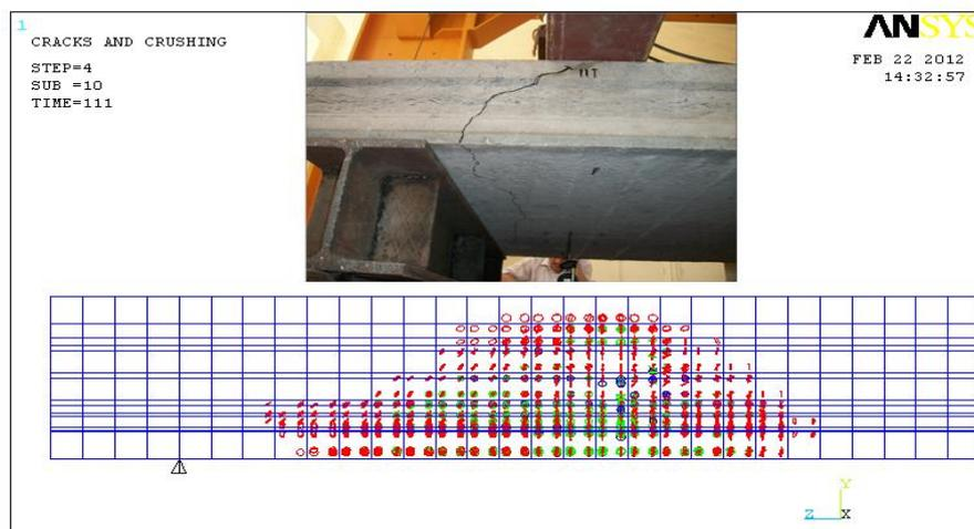
**Fig. 13:** Crack pattern and failure modes for Exp. and FEM slab SA.
