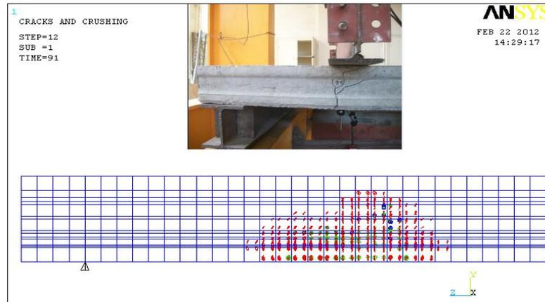
**Fig. 14:** Crack pattern and failure modes for Exp. and FEM slab SB.
